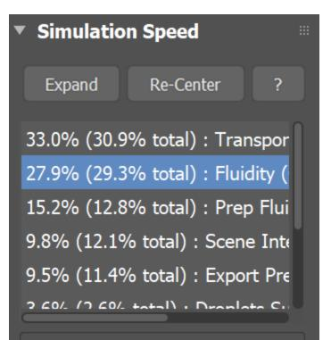
To speed up the simulation the most, reduce the Steps Per Frame option as much as possible. Keep it high only if there is fast movement of the fluid or obstacles in the simulator, or if you need stronger viscosity, or if the liquid needs to be smoother.
