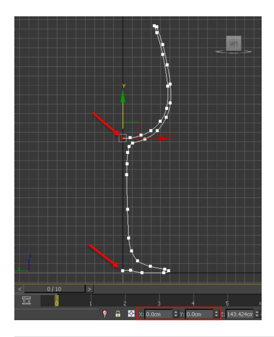
Next, add the  ${\bf Lathe}$  modifier by selecting it from the  ${\bf Modifier}$   ${\bf List}.$  This will create the cup geometry.
