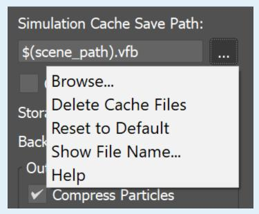
Browse - Opens a dialog where you can select where the simulation caches will be written to. The filename you type in must contain # signs so each simulation frame will be written to a differently numbered file. Also, you can choose between two file formats - AUR and VDB cache files. In order to write the simulation caches to VDB in the default simulation path, you can just edit the Simulation Cache Save Path to \$(scene\_path).vdb.
