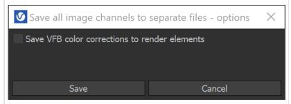
Save VFB color corrections to render elements – When enabled, all color corrections are saved to the render channels (as opposed to only the RGB and effectsResult channels).
