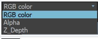
This dropdown gives access to render elements rendered for the scene. The selected render element is displayed in the VFB. By default, the RGB and Alpha render elements are available. Any additional render elements that have been added to the scene also appear in the drop-down.
