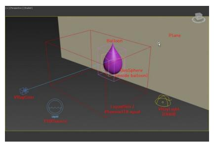
Since the simulated balloon geometry has no thickness, we can't use it as-is in the Phoenix simulation.
