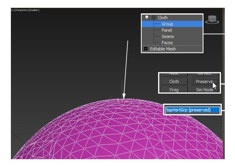
Change your mouse selection mode to Paint Selection. You can control the size of the brush by Right-Mouse-Button clicking on the Paint Selection icon and editing the **Paint Selection Brush Size** parameter from the General tab.
