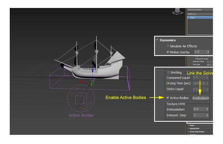
When you start the simulation, the Active Body Solver will create a duplicate of your object and keyframe its Position and Rotation for every single frame.
