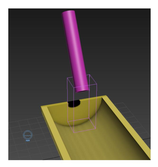
In this case, the Grid that was automatically created is not large enough to encompass a simulation of water flowing down the trough.
