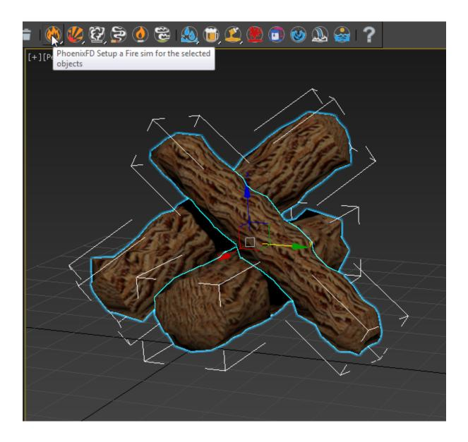
The Fire Quick Simulation button creates three objects in the scene and sets up their parameters for a fire simulation:
