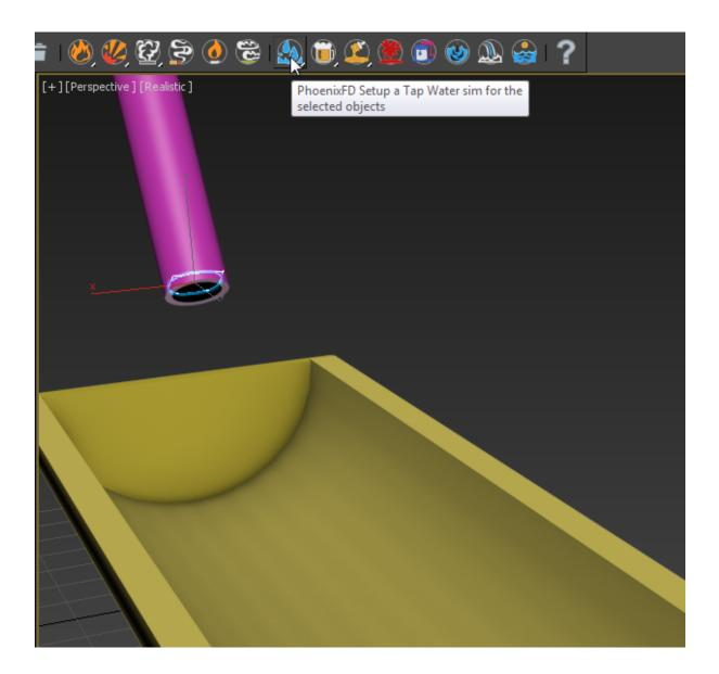
The Liquid Quick Simulation button creates two objects in the scene and sets up their parameters for a liquid simulation:
