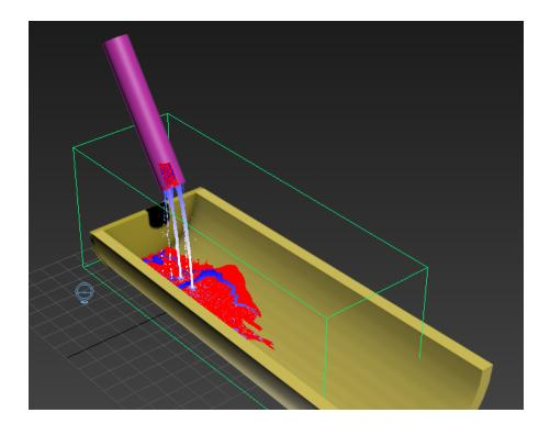
In a liquid simulation, you will see the liquid particles react to gravity and also get deflected or contained by any scene geometry they encounter, such as the trough. This collision detection occurs by default, even though you have not specifically designated the trough geometry as a deflector or collision object.
